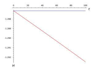
Dependence of energy H on time for approximate solutions found using our algorithm (blue) and the rk4 scheme (red).
