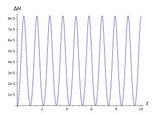
Dependence of energy increment  $\Delta H$  on time for approximate solution founded by midpoint scheme **without** auxiliary variables.
