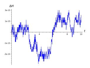
Dependence of energy increment  $\Delta H$  on time for approximate solution founded by midpoint scheme with auxiliary variables.
