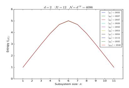
The figure presents the values of entropy  $S_2(\rho_A)$  computed in the ontic basis for the decomposition  $\mathcal{N}=2^{12}$ . Data for subsystems of all possible sizes, computed for ten randomly generated ontic vectors, demonstrate the following features:
