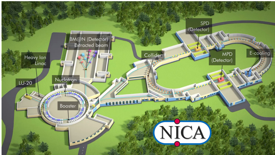
Scheme of the NICA complex with MPD, SPD, BM@N experiments.
