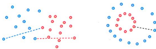
Figure 2.16 The Hausdorff distance is determined by the point in A with the largest distance to the closest point in B (and vice versa).
